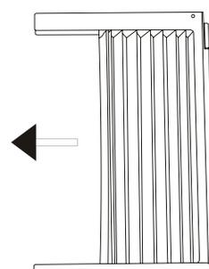
A. Place unit on floor, a bench or a table. Hold the Accordion Panel in one hand and gently pull back the center to free the open end. See Fig.1
